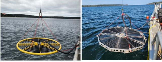
FIGURE 2: CANADIANPOND UPWELLING SYSTEMS (SALMOAIR® (LEFT) AND OCTOAIR-60 (RIGHT))
