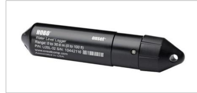
FIGURE 10: WATER LEVEL AND TEMPERATURE LOGGER
